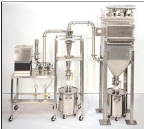
Model 8 Micro-Jet System designed for continuous processing of bulk pharmaceutical at a rate of 50 lbs/hr.
